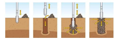
Figure 1: Dry – top - feed method process schematic( Taube, 2001).
