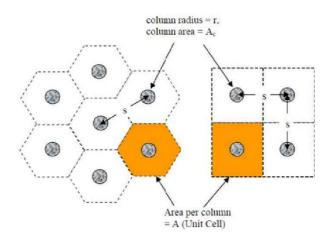
Figure 4:Plan of stone column, Triangular pattern (left) and square pattern (right).(Cabe, 2007).
