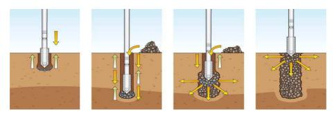
Figure 3: Wet - top - feed method process schematic (Taube, 2001)
