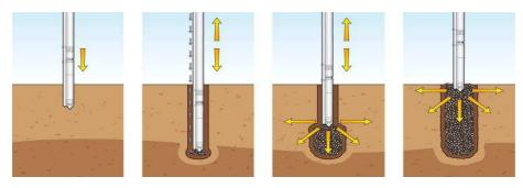
Figure 2: Dry – Bottom - feed method process schematic (Taube, 2001).
