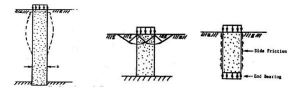
A. long stone column with firm or floating support (bulging failure)
